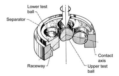
Perhaps the key objection to this geometry is that the load at each point of contact between upper ball and supporting ball is statically indeterminate, whereas with three supporting balls, the load is fully determinate.
