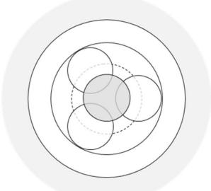
The solution adopted by numerous researchers (including Cameron-Plint Tribology in the 1980s) is to separate the three supporting balls with a cage. This thus replaces the sliding contacts between the balls with a sliding contact at approximately half the speed between ball and cage. This has two beneficial effects:
