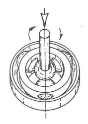
As well as rolling four-ball test geometries with cages or "separators", some researchers have also adopted a rolling five-ball test geometry in which the upper ball is supported on four lower balls.
